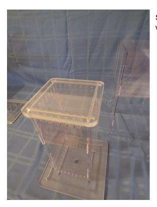
Set the smaller lid D on the interior box so the box walls fit in the grooves.
