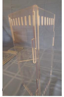
Take one A1 piece with the long slot closest to the shorter edge at the top, insert hooks from an A2 piece and slide to form a corner of the box. Repeat to form the remainder of the box.
